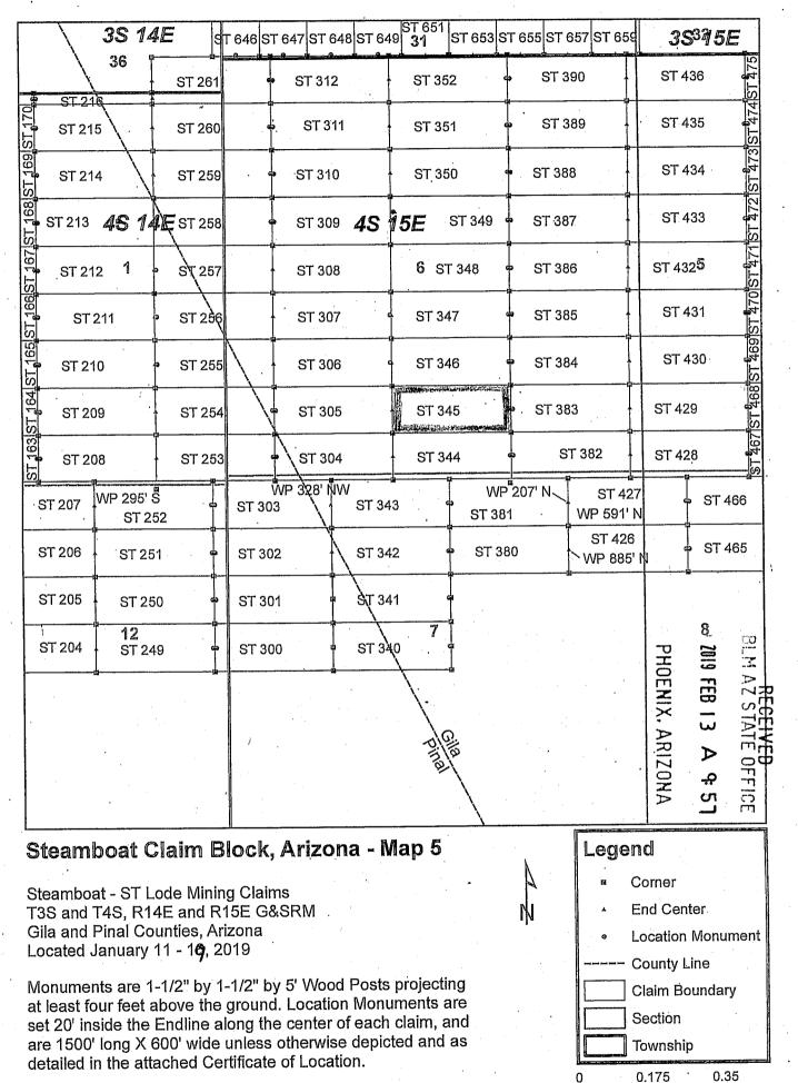
is tied to the northeast corner of Section 28, Township 3S, Range 15E, G&SRM, Gila County, Arizona, its distance as shown on the attached Certificate of Location. Bearings and distance are grid north.
