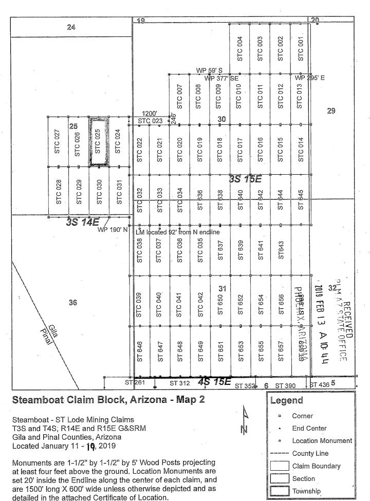
is tied to the northeast corner of Section 33, while the location monument of claims ST 600 - ST 677 and STC 001 - STC 042 is tied to the northeast corner of Section 28, Township 3S, Range 15E, G&SRM, Gila County, Arizona, its distance as shown on the attached Certificate of Location. Bearings and distance are grid north.
