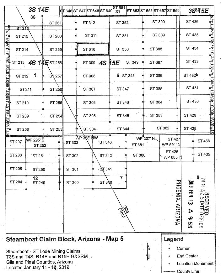
Monuments are 1-1/2" by 1-1/2" by 5' Wood Posts projecting at least four feet above the ground. Location Monuments are set 20' inside the Endline along the center of each claim, and are 1500' long X 600' wide unless otherwise depicted and as
