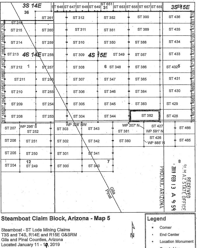
Monuments are 1-1/2" by 1-1/2" by 5' Wood Posts projecting at least four feet above the ground. Location Monuments are set 20' inside the Endline along the center of each claim, and are 1500' long X 600' wide unless otherwise depicted and as detailed in the attached Certificate of Location.
