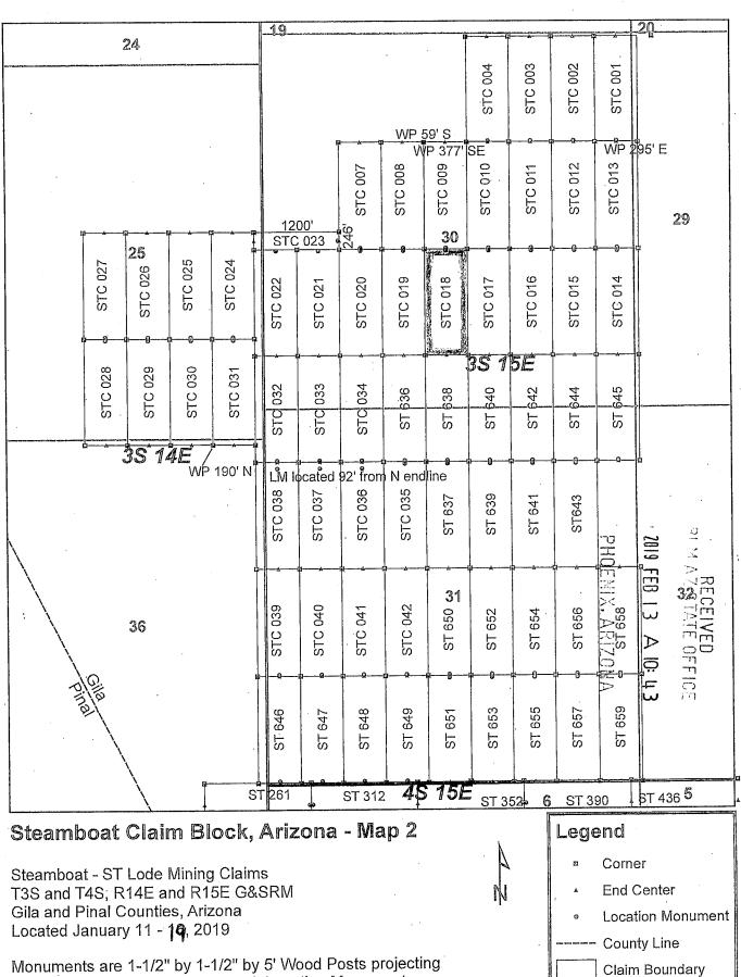
Monuments are 1-1/2" by 1-1/2" by 5' Wood Posts projecting at least four feet above the ground. Location Monuments are set 20' inside the Endline along the center of each claim, and are 1500' long X 600' wide unless otherwise depicted and as detailed in the attached Certificate of Location.
