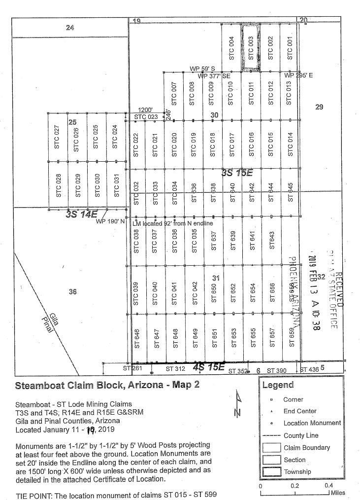
is tied to the northeast corner of Section 28, Township 3S, Range 15E, G&SRM, Gila County, Arizona, its distance as shown on the attached Certificate of Location. Bearings and distance are grid north. Any overlap onto pre-existing lode claims, or Private Land,
